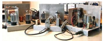
Chassis view of a replica Kričač transmitter unit (left), modulator unit (centre) and mains power unit (right), constructed by Janez Červek.
